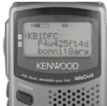
**Figure 5** — The TH-7DA(G) displays an APRS packet from KB1DFC. The text indicates that KB1DFC is running 4 W power, is 425 feet above sea level and is using a 4 dB omnidirectional antenna.
